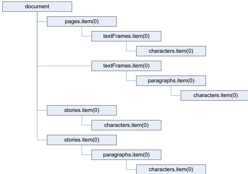
For any text stream object, the `parent` of the object is the story containing the object. To get a reference to the text frame (or text frames) containing the text object, use the `parentTextFrames` property.
