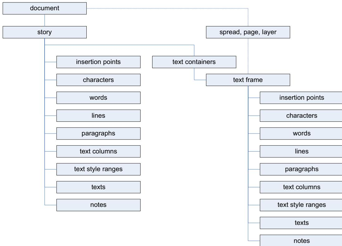
There are many ways to get a reference to a given text object. The following diagram shows a few ways to refer to the first character in the first text frame of the first page of a new document:
